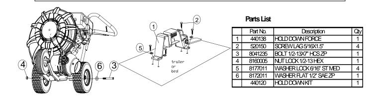
To use the Hold Down, simply rest the bolt mounted previously behind the tire in the slot area that the pin will retract. Using your foot press the lever and lower the blower into the Hold Down unit gently until it rests at the bottom of the slot. To release simply reverse order used to Hold Down unit.
